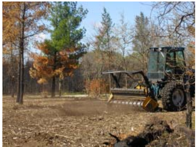
A May 26th demonstration helped landowners who had forests burned in the May 5th Cottonville Fire learn about salvage of their charred timber. The event included a demonstration of a timber mulcher to grind standing charred trees that were too small to be salvaged.
